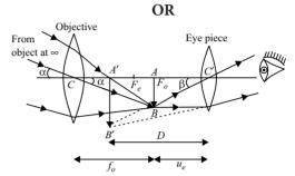
Here,  $f_o = 15 \text{ m} = 1500 \text{ cm}$  and  $f_e = 1.0 \text{ cm}$  Angular magnification by the telescope in normal adjustment
